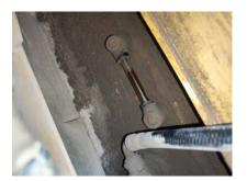
9.2 Inspect hydraulic cylinders for leaks and security
