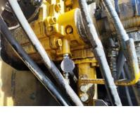
9.5 Check Pilot Accumulator operation as per OEM Maintenance Procedure -Test Boom Down Functionality with engine off
