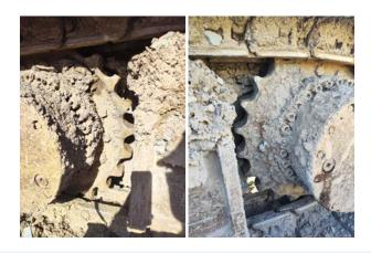
11.7 Inspect track frame for cracks, lose or missing hardware
