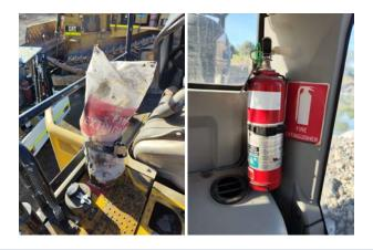
5.5 Check all fire extinguishers are correctly charged
