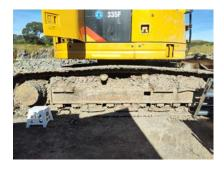
11.3 Inspect tracks for loose/missing bolts
