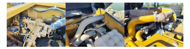
6.5 Inspect exhaust system for signs of leaks, loose bolts or missing clamps
