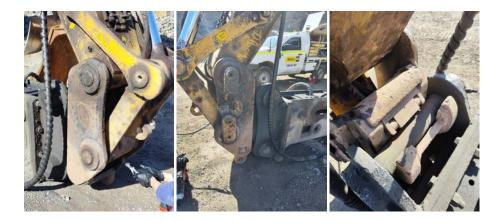
12.6 Inspect bucket condition – cracks, wear, damage, mounts
