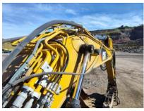
9.4 Inspect hydraulic pump condition, leaks, security
