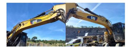
12.4 Inspect stick condition – cracks, missing clamps, damaged pipes, excessive movement, lubrication
