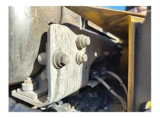
6.6 Inspect turbo for security and signs of leaks
