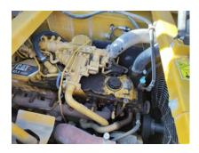
6.4 Inspect engine components for missing clamps
