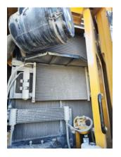
7.4 Check cooling system for signs of leaks
